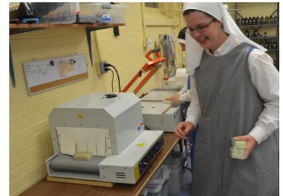
*The handmade soaps are now wrapped using the Clamco Sealer and run through the Clamco Model 61513 Heat Shrink Tunnel.*
