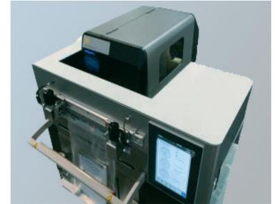
*Truly a next-generation automatic poly bagger, the R785 is the first all-electric bagger that offers an optional, integrated label printer applicator. This off the shelf industrial labeling solution prints and applies a label. As the label printer applicator works with direct thermal labels, as well as thermal transfer, there is no need for any printer ribbon. Custom pre-printed labels with high color graphics can also be used, for a retail customer experience that greatly enhances the brand.*
