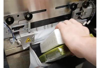
The Rollbag R785 bagger can be equipped with a range of options, printers, and feeding devices to maximize and automate virtually any packaging process.
