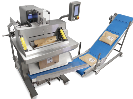
Rollbag R3200 configured to label, fill, & seal curbside recyclable paper mailers.
