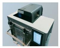
Truly a next-generation automatic poly bagger, the R785 is the first all-electric bagger that offers an optional, integrated label printer applicator. This off the shelf industrial labeling solution prints and applies a label. As the label printer applicator works with direct thermal labels, as well as thermal transfer, there is no need for any printer ribbon. Custom pre-printed labels with high color graphics can also be used, for a retail customer experience that greatly enhances the brand.
