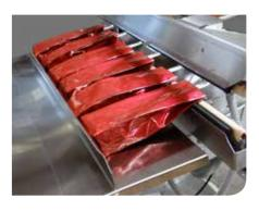
The Coffee Pac Express (pictured above) is our high production floor model vacuum sealer. Like our other nitrogen gas flush vacuum sealers, the Coffee Pac Express features a particle ejection system to clear the vacuum lines of coffee debris after every vacuum cycle.
